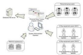
Polimaster Dose Tracking System is intended to provide acute dose information for the personnel and operators, working with the X-ray scanning equipment.
