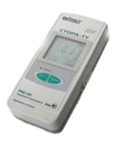
The modified device «STORA-TU» is smaller and has a modern damp and dustproof body (IP-54). Measurement units, measurement errors, alarm threshold level and real time are simultaneously displayed on a large liquid crystal display (LCD) with a luminescent backlight. Besides, the LCD displays a battery status symbol and a twelve-segment indicator of registered radiation intensity.
